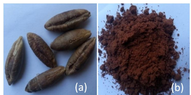
Figure 2 (a) Date palm seeds and (b) Particles of date palm seeds powder (0.2-0.4mm).
