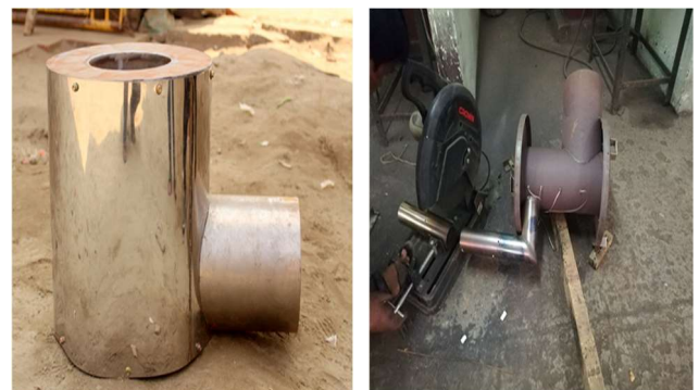
Fig. 1. Construction of Biomass Cook Stove.
