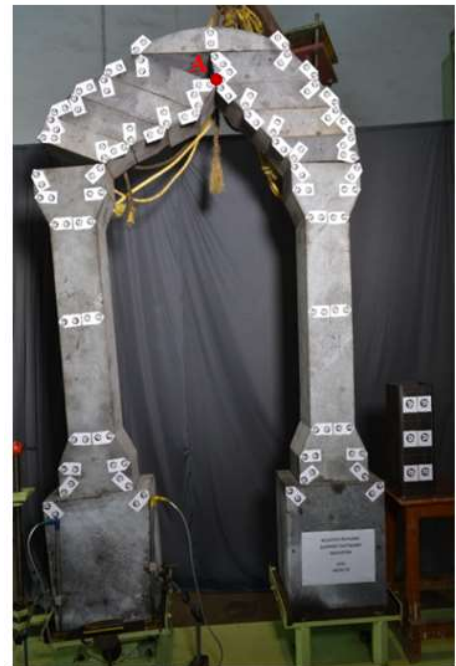
Figure 8: Corbel arch in the verge of collapse at an input outward rotation of 4°
