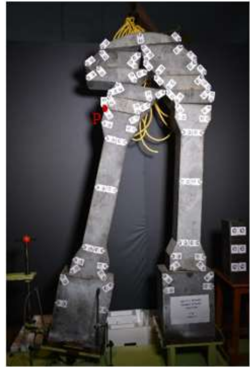
Figure 11: Corbel arch in the verge of collapse at 12.5 ° input inward rotation
