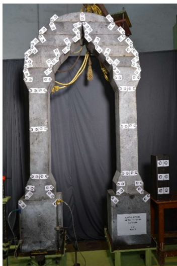
Figure 4: Test specimen with coded target markers
