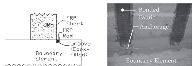
Fig. 1. GFRP laminate detail (Carney P. and Myers J. J., 2005)
