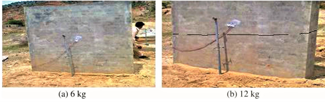
Fig. 26. Post-test view of URM walls tested for different explosive loads by Ahmad S. et al. (2014) [3]: (a) 6 kg, and (b) 12 kg
