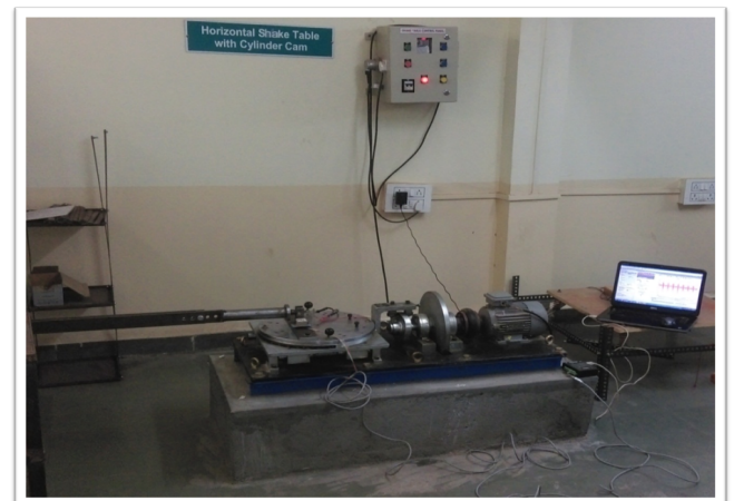
Figure 6: Experimental Setup of MR damper testing process.
