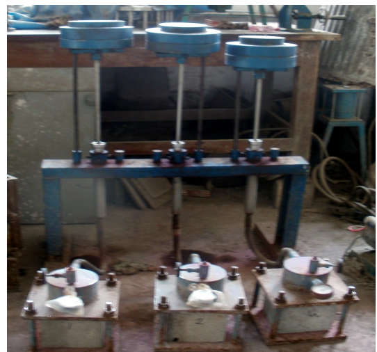
Fig. 2. Water Permeability Test Apparatus in IEST
