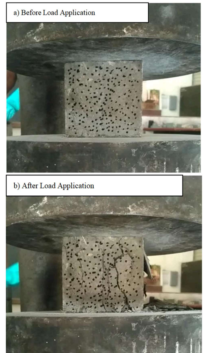
Fig. 9: Speckled pattern marked cube (a) before and (b) after applying load for control mix.
