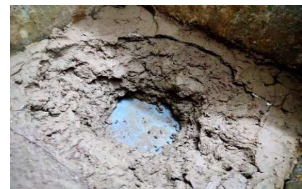
Fig 4.10: Actual failure plane observed after complete pull out test on belled pile.
