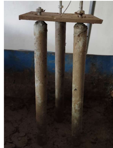
Fig 3.2: Triangular pattern arrangement with 3 cylindrical piles (2x1)
