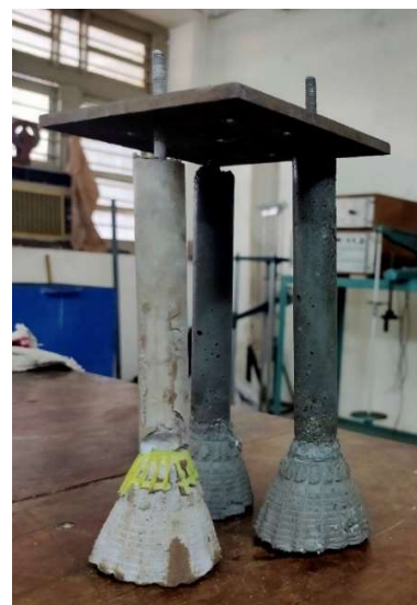
Fig 3.3: Triangular pattern arrangement with 3 belled piles (2x1)
