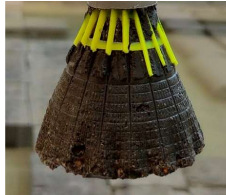
Fig 3.1: Belled portion of a belled pile
