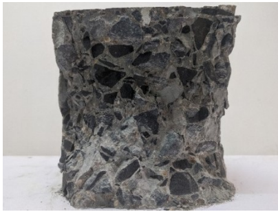
Fig. 4 Typical failure of M80 concrete without fibre reinforcement
