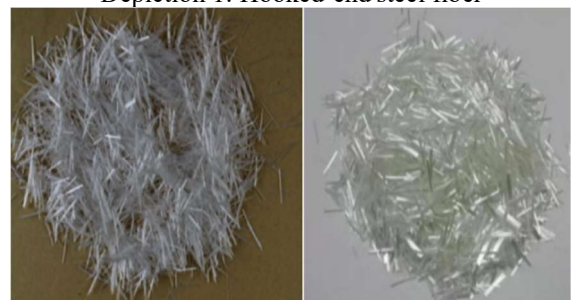
Depiction 2: Cement-fil anti-crack alkaline resistant glass fibers
