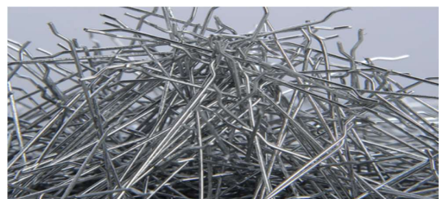
Depiction 1: Hooked-end steel fiber
