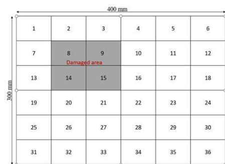
Fig. 2. Schematic diagram of the rectangular FRP plate with induced damage location.
