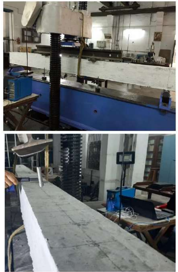
Figure 2: Static and Dynamic Testing of RC Beam
