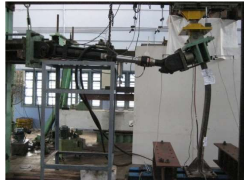
Fig. 9. Failure mode - Global buckling of column C3-0.8P
