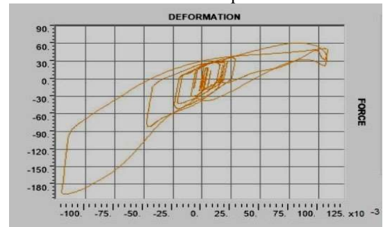
fig.f Force displacement graph for Friction Pendulum isolator Erzinkan earthquake
