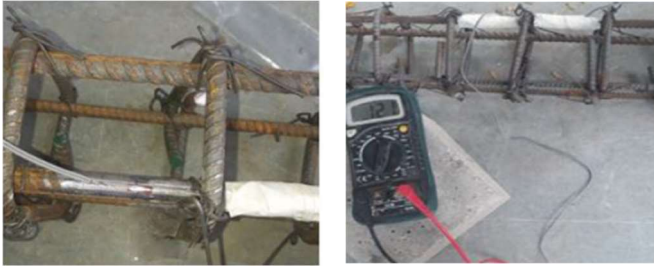
Fig 5. Installation and strain gauge resistant measurement
