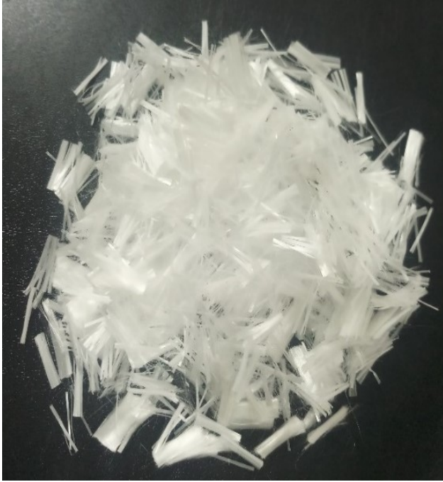
Fig.6. Fibrillated mesh type recycled plastic fiber
