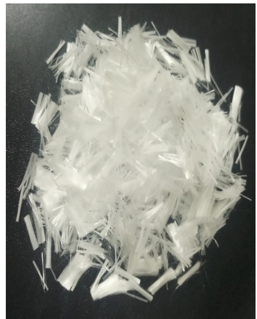
Fig. 1. Fibrillated mesh type recycled plastic fiber
