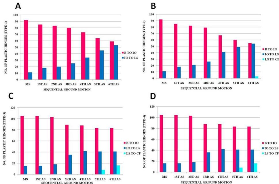
Fig.8 Number of hinges pattern under sequential ground motion (Case2) for A. (Type-1), B. (Type -2), C. (Type-3), and D. (Type -4)
