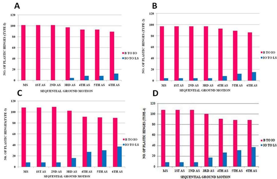
Fig.7 Number of hinges pattern under sequential ground motion (Case1) for A. (Type-1), B. (Type -2), C. (Type-3), and D. (Type -4)
