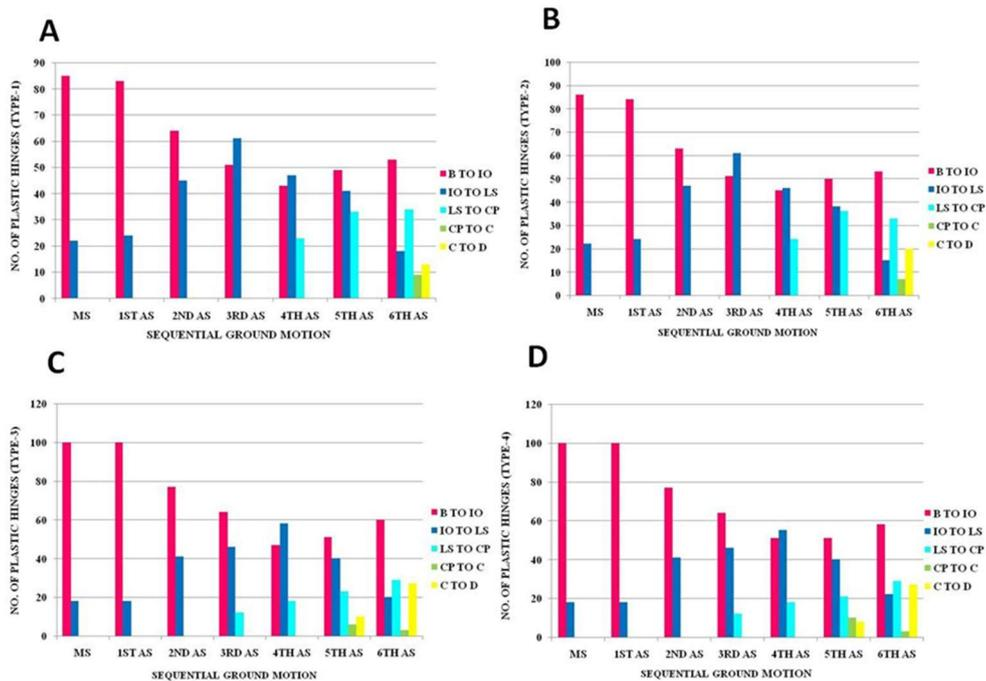
Fig.9 Number of hinges pattern under sequential ground motion (Case3) for A. (Type-1), B. (Type -2), C. (Type-3), and D. (Type -4)
