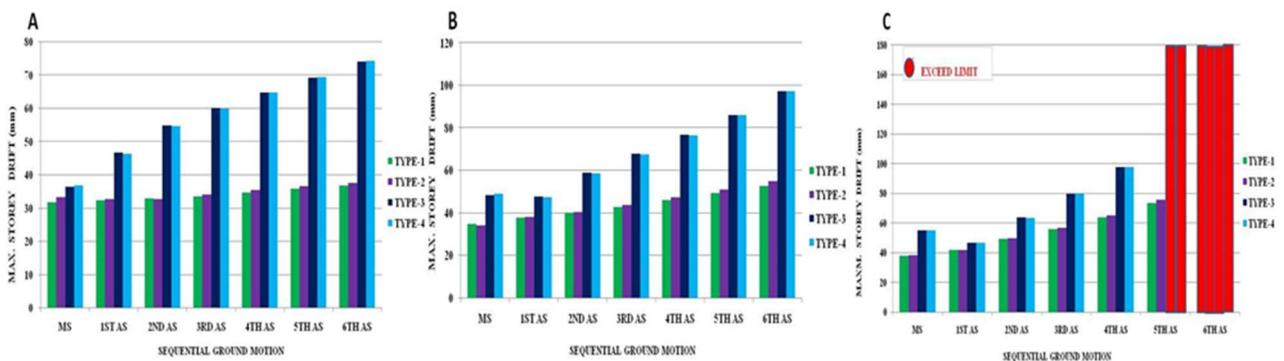
Fig.5 Maximum transient storey drift of different type building (Type-1, Type-2, Type-3, Type-4), seismic sequence for A (Case1), B (Case2), C (Case3)
