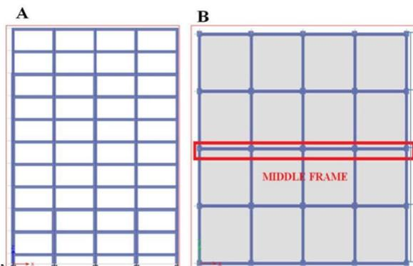
Fig. 1 A Elevation detail of (G+10) storey RC Regular Frame; B Plan view of the building
