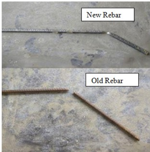
Fig. 8. Typical broken rebars after tensile test
