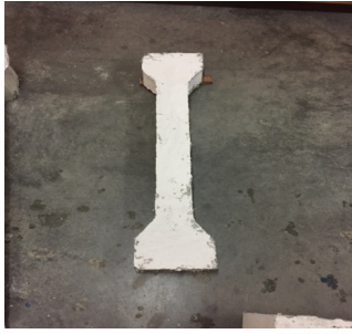
Fig.2. HPFRCC Short column specimen before testing
