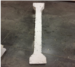
Fig.3. HPFRCC Slender column specimen before testing
