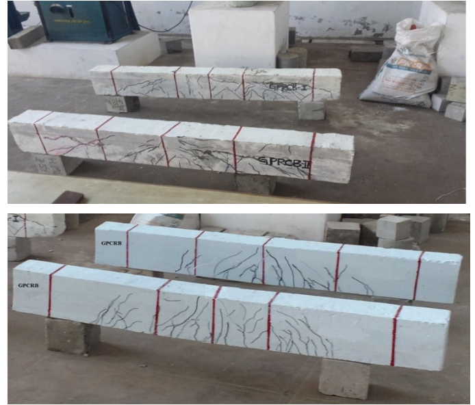
Fig.5 Mode of failure of GPC specimens
