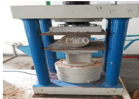
Figure.13 Split Tensile Test
