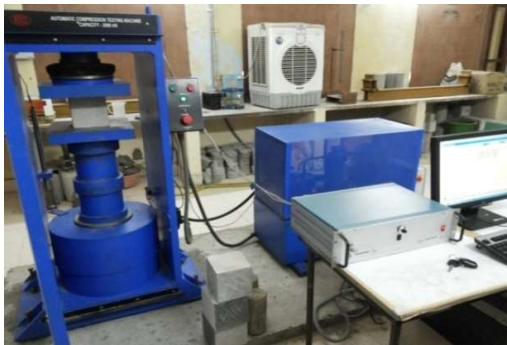
Figure.12 Compression Testing Machine
