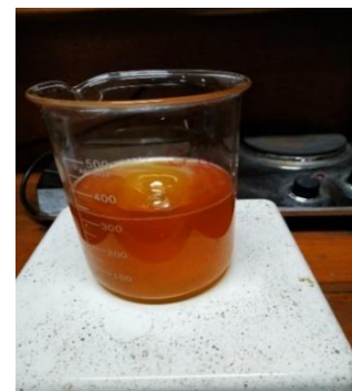
Fig. 3. Transesterification Reaction Occurring in the mixture of the Waste Cooking Oil and the Methyl-Oxide Solution.
