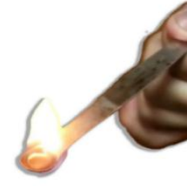
Fig. 6. Burning test of the produced biodiesel.
