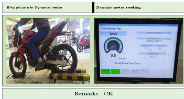
Figure 14. Front brake force test.
