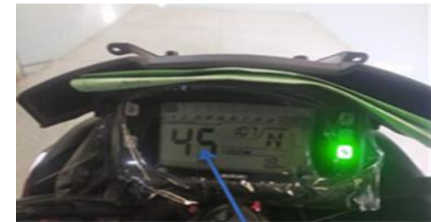
Figure 13. Motorcycle meter calibration test
