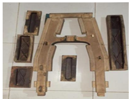
Figure 7. Swing arm Wood pattern.
