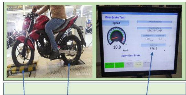
Figure 15. Rear brake force test.
