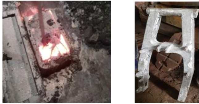
Figure 8. Swing arm casting.
