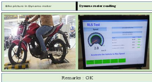
Figure 16. Top speed test.
