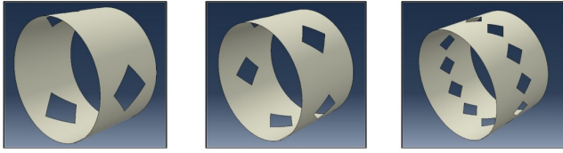
Fig. 4. Modelling of diamond-notched shells in ABAQUS/Explicit®
