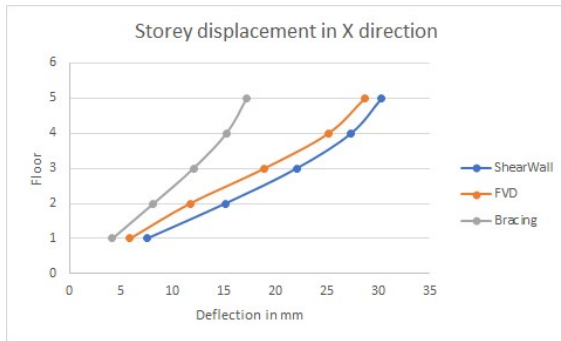
Fig 13: Comparison of storey displacement for the three retrofit strategies (optimal configuration)
